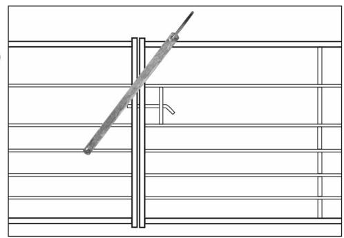
For 50mm (2" Wide) Steel Gates Including Bolt & Nylock Nut Overall Length 34" (860mm) Loop Length 6" (155mm)
